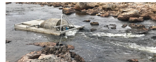
A rotary screw trap in the River Spey to safely catch and count young salmon as they swim downstream.
